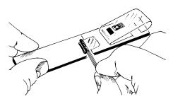
After mixing the adhesive in accordance with this bulletin, use scissors to snip off one corner of the bag. Squeeze the adhesive out of the package onto a cleaned surface, preferably a glass plate. Apply a liberal coating of the adhesive to the specimen or the gage backing using a glass or plastic stirring rod. Smooth to a uniform thickness over the desired area. The adhesive film should be just thick enough to cover the gaging area without bubbles or voids.
