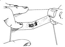
Remove the gage/tape/terminal assembly by peeling tape at a shallow angle (about 45 deg) and transferring it onto
