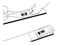
Lift one end of the tape at a shallow angle to surface (about 45 degrees) until the gage and terminal are free of the specimen surface. Tuck loose end of the tape under and press to surface so the gage lies flat with the bonding side exposed.
