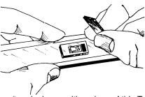
Overlay gage/terminal area with a piece of thin Teflon sheet (TFE-1). If necessary, anchor Teflon in position with a piece of Mylar tape across one end.
