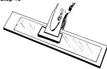
Apply force by spring clamp or dead weight until a clamping pressure of 15 psi (105 kN/m2) is attained. Take special care in making sure the clamping pressure is
