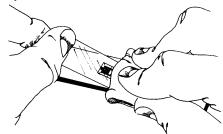
Lift the tucked-over end of tape and bridge it over the adhesive at approximately a 30-degree angle. With a piece of gauze, slowly make a single wiping stroke over the gage/tape assembly, bringing the gage back down over the alignment marks on the specimen. Use a firm pressure with your fingers when wiping over the gage, since the adhesive is quite viscous. A very thin layer of adhesive is desired for optimum bond performance.
